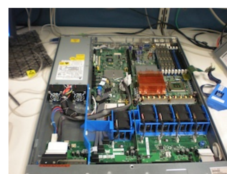
Intel QuickIA prototype: Intel Xeon E5450 (high performance) + Intel Atom N330 (low power)
